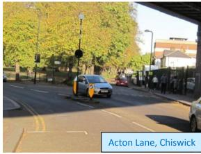
It is possible to install narrow waiting restriction double and single yellow lines (ie 50 mm width in place of 100 mm wide lines). These are perfectly clear to drivers and have been installed in some new Reading schemes (eg Vastern Road).
